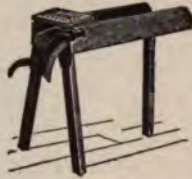
Fig. 78. A lever cutter.
